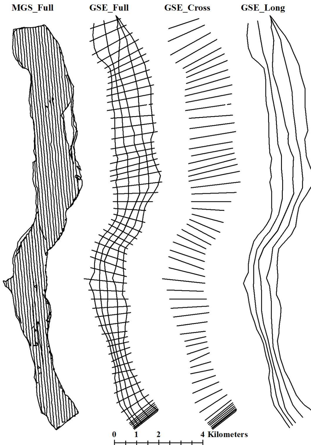
**Figure 1: Track lines for four survey designs analyzed on Conowingo Pond.**
